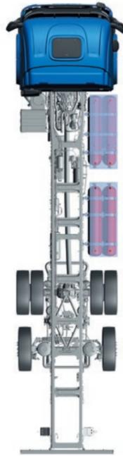
CNG tanks on the right side, available in combination with, on the left side:
