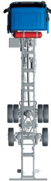
CNG tanks behind the cab, available in combination with:
