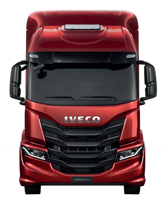
AT440S43TZ/P ON – 6x4 Truck Tractor, Pneumatic Suspension
