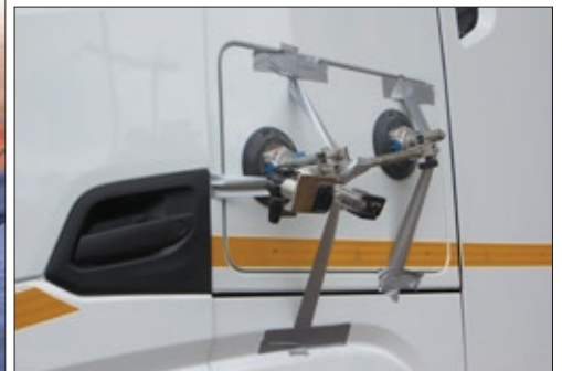
▲ A high definition GoPro camera was fixed to the cab to track the wheel and tyre during the test.
