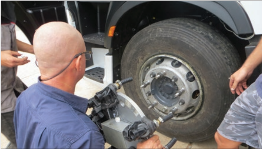
▲► The deflation device being fitted to the rim and then tightly fastened. The device itself was designed and made specifically for this project which, in itself, was a feat of engineering excellence with no margins for error.
