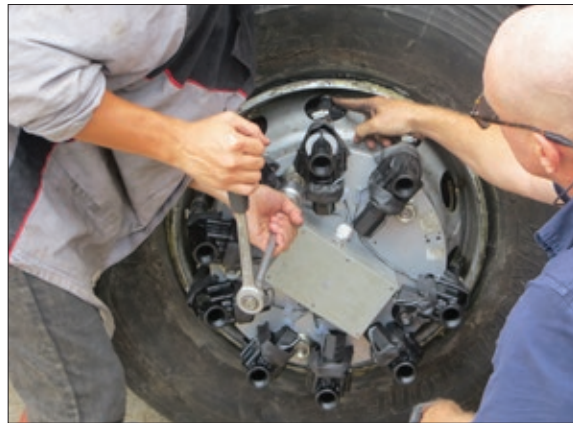
▲► The deflation device being fitted to the rim and then tightly fastened. The device itself was designed and made specifically for this project which, in itself, was a feat of engineering excellence with no margins for error.
